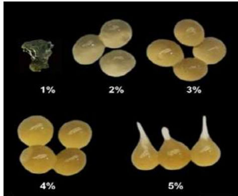
Figure 1. Effect of sodium alginate concentration (in 100 mM calcium chloride) on the size, shape and consistency of beads (Gantait et al., 2015)
